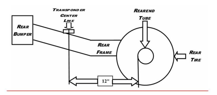
Transponder mounting bracket will be installed on the inside of the left rear frame rail.
