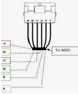
(A), (B), (C), (D), (E) and (F) to the 8170 Connector.(G) Maximum 36" (H) Maximum 12" (quick-connect plugs recommended)
